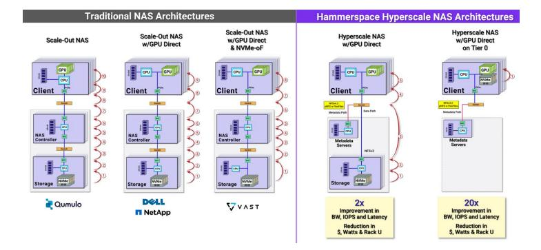
A traditional Scale-out NAS design requires a NAS controller in the storage system. There are two key areas where this causes issues:
