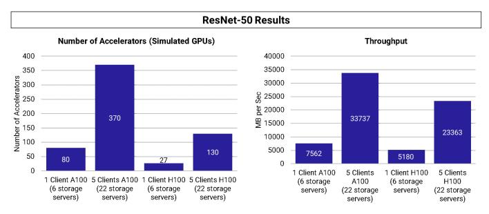
In the ResNet-50 image classification workload simulation, a Hammerspace system with 22 flash-based Linux storage servers (LSSs) drove 370 simulated A100 GPUs and 130 simulated H100 GPUs to > 90% utilization, delivering 33.7GB/s and 23.3GB/s aggregate read performance, respectively.
