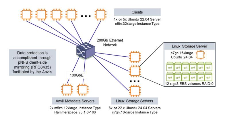
The Hammerspace system consisted of two redundant Anvil metadata servers in an active/passive configuration and up to 22 Linux storage server (LSS) nodes. The Anvil servers are responsible for metadata operations and cluster coordination tasks, while the LSS nodes serve test data using associated solid-state EBS volumes storage devices. Single-client tests used six LSS nodes, and multiple-client tests used all 22.
