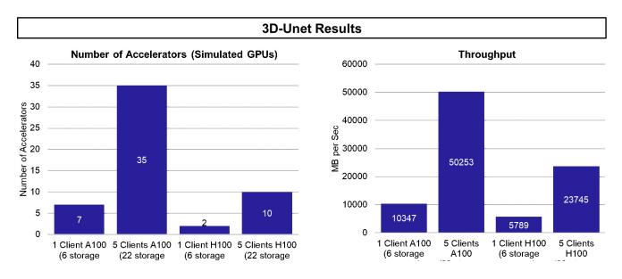
With the 3D-Unet simulated image segmentation workload, this system drove 35 simulated A100s and 10 simulated H100s, delivering 50.3GB/s and 23.7GB/s, respectively.
