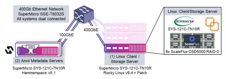
Configuration 2b is used to demonstrate Tier 0 performance. Two redundant active/passive Anvil metadata servers are responsible for metadata operations and cluster coordination tasks. The client in this test has two roles. It runs the benchmark code as usual, but is also the storage server, serving the test data from internal ScaleFlux CSD5000 Computational Storage NVMe drives. No computational storage features of the ScaleFlux drives were used in this test.
